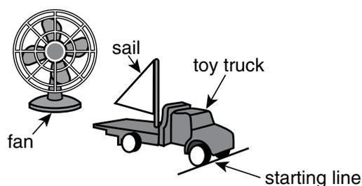
Jonah switched on the fan. The moving air pushed against the sail, causing the truck to begin to move. The truck moved along the floor before slowing and coming to a stop. Jonah performed 2 investigations to study the motion of the truck.
